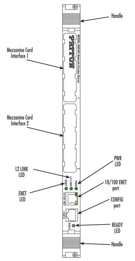
Figure 2. Model 6081RC front panel
